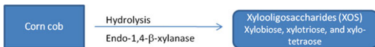
Fig. 2.4 Commercial production of xylooligosaccharides, which are most commonly from corncobs but also can be extracted from hardwood. Xylooligosaccharides are extracted by hydrolyzing xylans in the starting material using endo-1,4- \beta -xylanase
