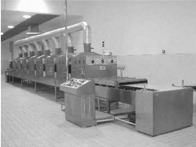
**FIGURE 1** Automated microwave drying processing line to produce nutritional egg flakes. (Courtesy of Taiyo Kagaku.)
