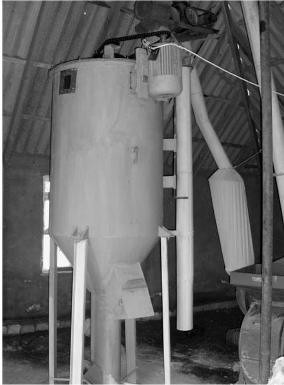
**Fig. 5.1.** A small mix-mill for on-farm use.
